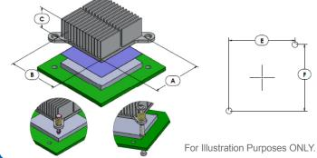
**NOTES:** 1) Dimension A is the length of the heat sink in the direction of the flow.
