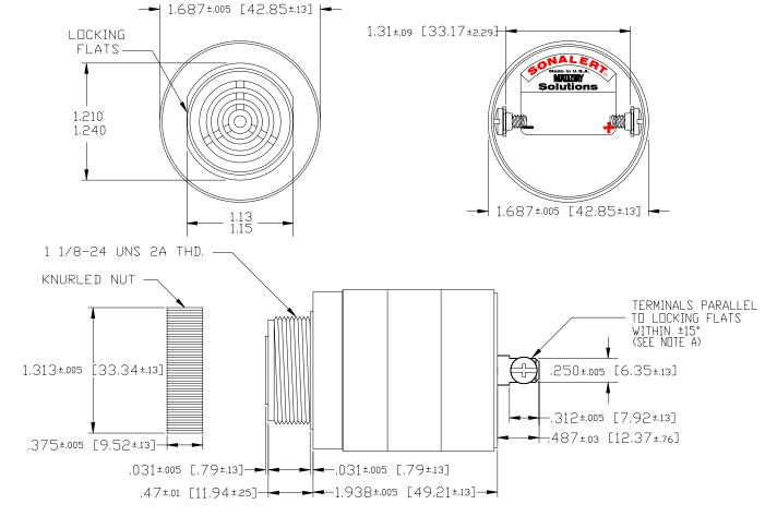
NOTE: MOUNTING- REMOVE BLACK PLASTIC NUT AND INSERT THREADED FRONT THROUGH 1.25" HOLE PUNCHED IN PANEL, IF ORIENTATION IS NEEDED, NOTE LOCKING FLATS ON DRAWING. SCREW NUT BACK ON.
