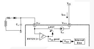
Figure 14. Startup Circuit
