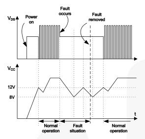
Figure 17. Auto-Restart Protection Waveforms
