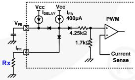
Figure 23. Peak Current Limit Adjustment
