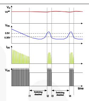
Figure 22. Burst-Mode Operation
