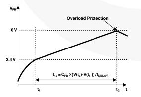
Figure 18. Overload Protection (OLP)
