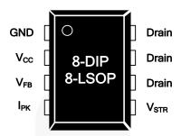
Figure 3. Pin Configuration
