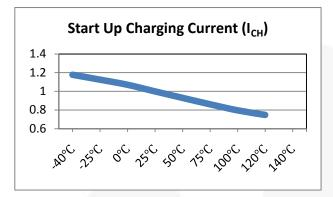
Figure 10. Startup Charging Current vs. Temperature
