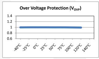
Figure 13. Over Voltage Protection vs. Temperature
