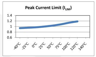
Figure 11. Peak Current Limit vs. Temperature
