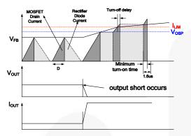
Figure 20. Output Short Waveforms (OSP)
