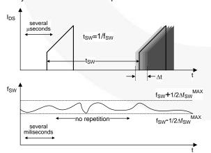
Figure 15. Frequency Fluctuation Waveform
