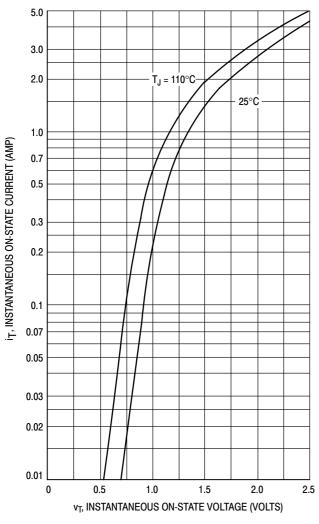
Figure 3. Typical Forward Voltage
