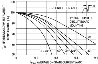
Figure 2. Maximum Ambient Temperature
