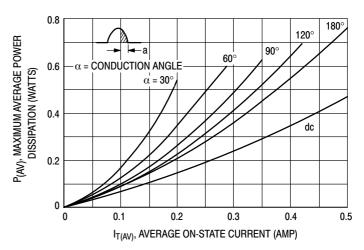
Figure 5. Power Dissipation
