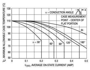
Figure 1. Maximum Case Temperature
