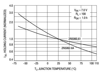
Figure 9. Typical Holding Current
