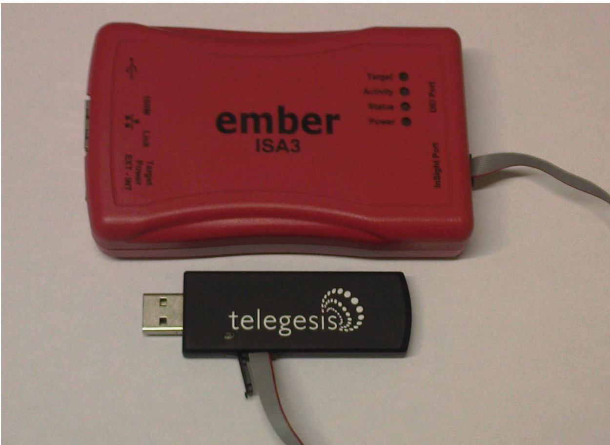
Figure 4: Connecting the ETRX357USB to the Ember ISA3
