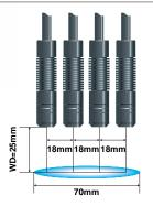
When high-intensity heads equipped with ANUJ6475S (cylindrical lens) are used with 18 mm pitches as shown in the figure, an entire linear area of approx. 70 mm wide can be reliably irradiated at 350 mW/cm<sup>2</sup> or higher intensity.
