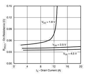
On-Resistance vs. Drain Current
