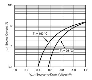
Source-Drain Diode Forward Voltage
