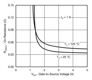
On-Resistance vs. Gate-to-Source Voltage
