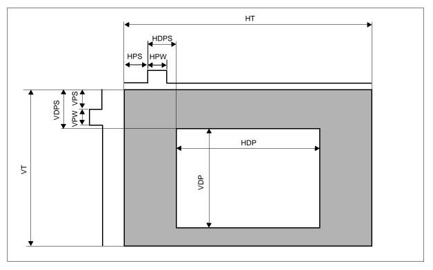
Figure 7-16: Generic TFT Panel Timing
