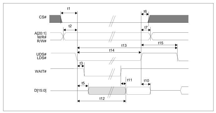
Figure 7-12: Direct/Indirect 68 Host Interface Read Timing
