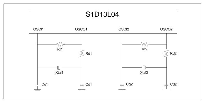
Figure 18-1: Recommended Crystal Oscillator External Circuit
