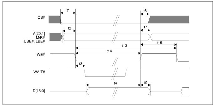
Figure 7-7: Direct/Indirect 80 Type 1 Host Interface Write Timing
