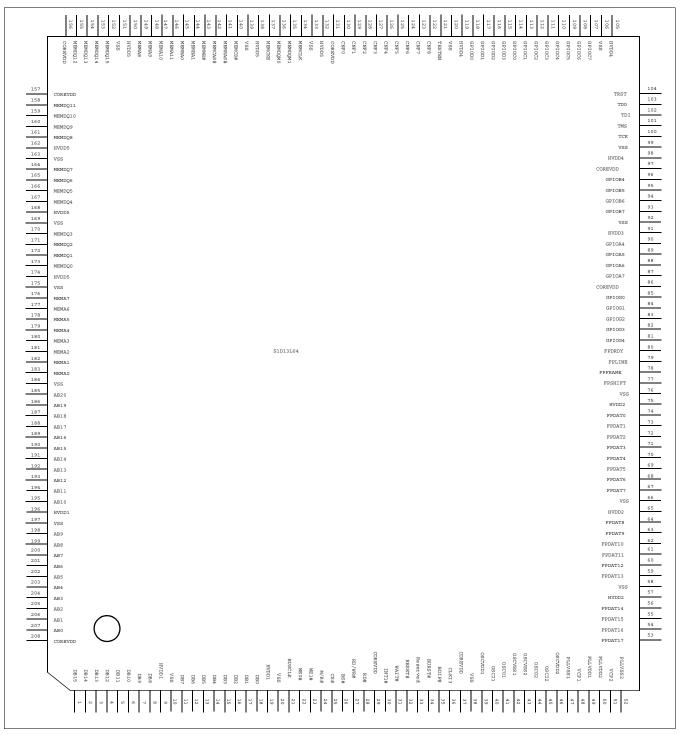
Figure 5-1: QFP22-208 Pinout
