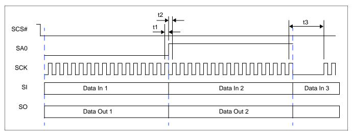
Figure 7-15: Serial Host Interface Burst Mode Timing
