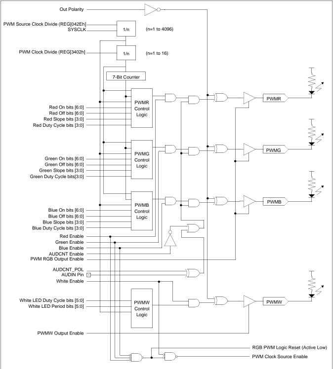
Figure 15-3: PWM Block Diagram
