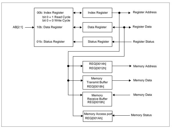
Figure 16-3: Indirect Interface Block Diagram
