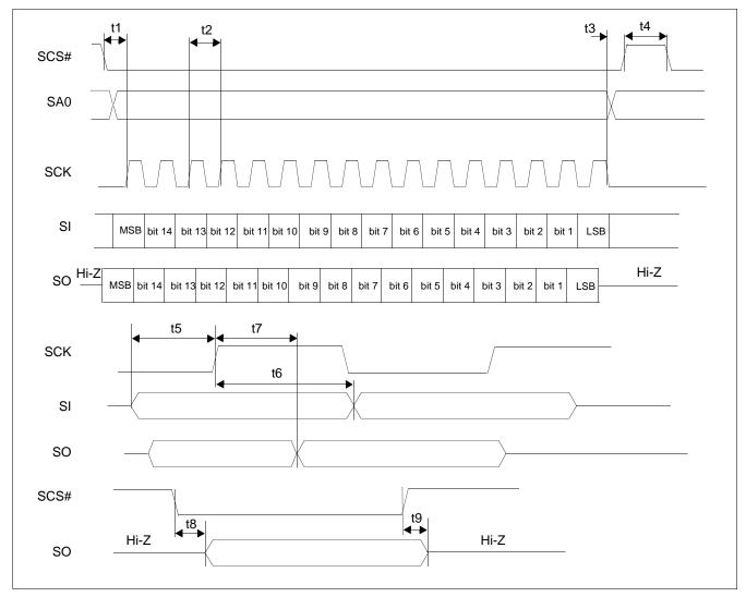
Figure 7-14: Serial Host Interface Timing for Data Valid on Rising Edge of SCK
