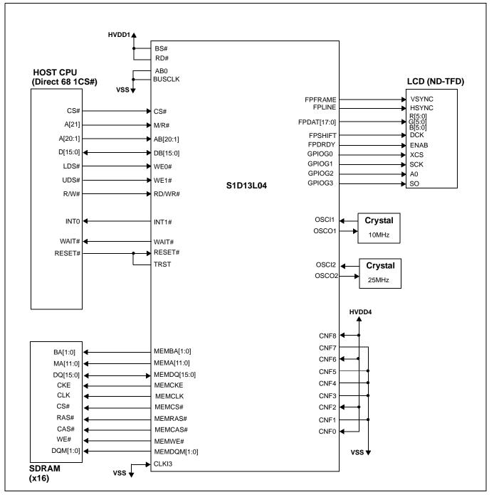
Figure 3-1: Example System Diagram
