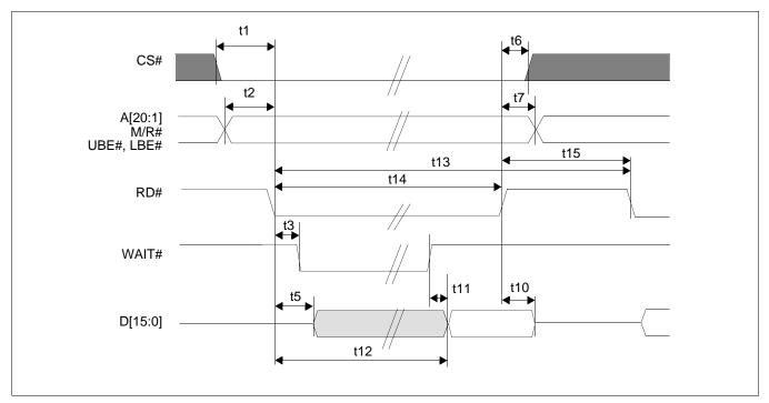
Figure 7-8: Direct/Indirect 80 Type 1 Host Interface Read Timing
