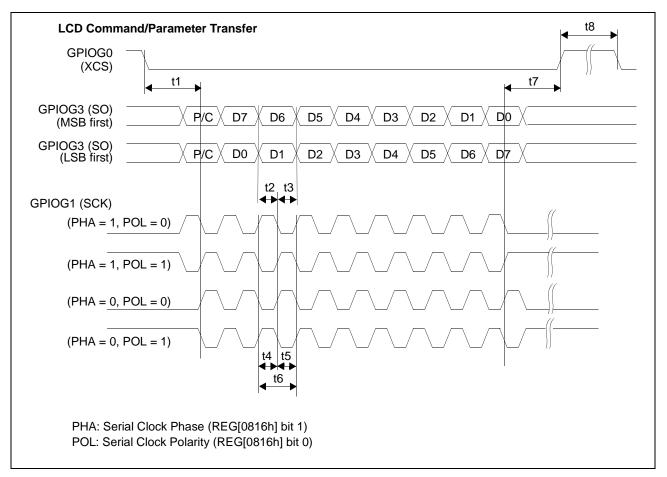
Figure 7-20: ND-TFD 9-Bit Serial Interface Timing
