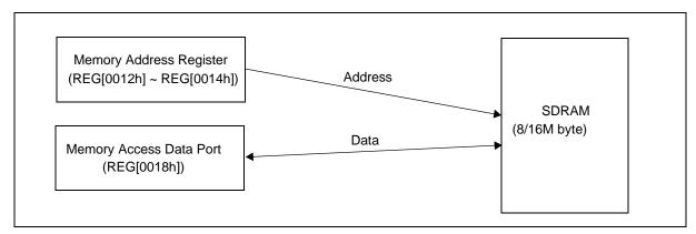
Figure 8-2: External Memory (Indirect Access)
