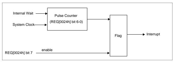
Figure 16-1: Host Read/Write Cycle Time-out Function
