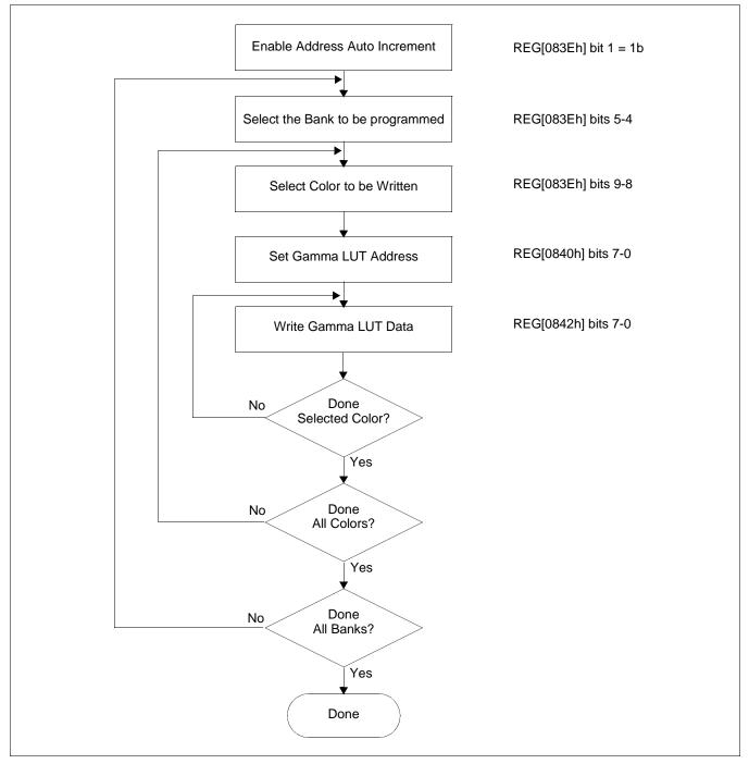
Figure 13-7: Gamma LUT Programming Flowchart
