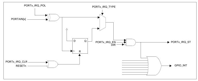
Figure 10-1: GPIOA and GPIOB Interrupt Logic
