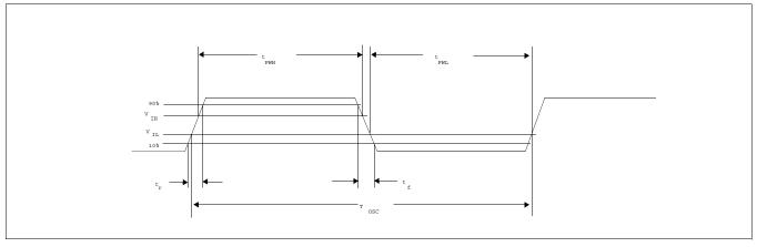
Figure 7-1: Clock Requirements for OSC1/OSC2/CLKI3/BUSCLK
