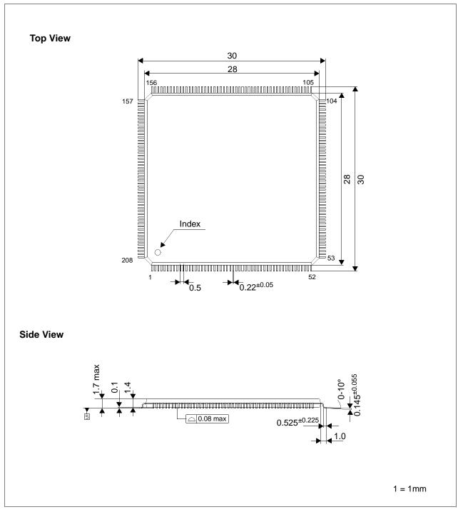
Figure 20-1: S1D13L04 QFP22 208-pin Package
