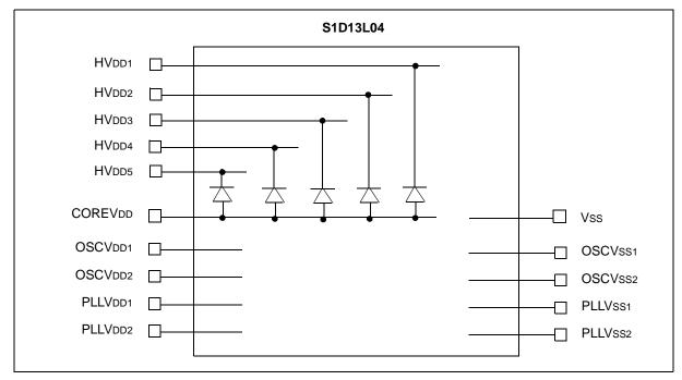
Figure 7-3: Internal Power Structure
