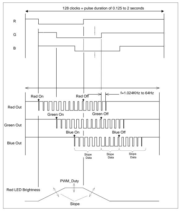
Figure 15-2: PWM Timing Diagram
