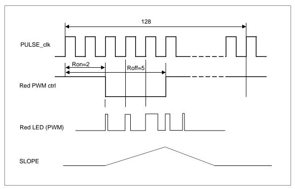
Figure 15-1: PWM Timing Example
