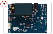
Insert the 9-V battery into the battery holder. Press firmly in place.
