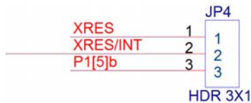
Figure 3-6. XRES/INT Selection Jumper
