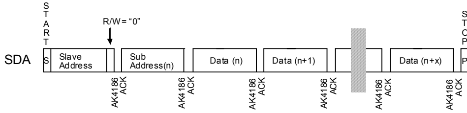
Figure 7. Data Transfer Sequence at the I 2 C-Bus Mode
