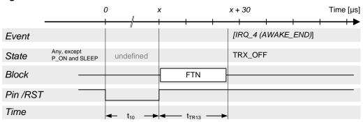
Figure 7-7. Reset Procedure.
