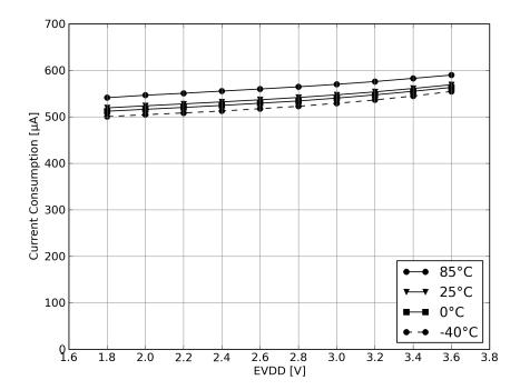
Figure 13-1. Current Consumption in P\_ON State.
