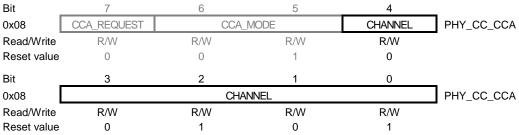
The register PHY\_CC\_CCA contains register bits to set the channel center frequency according to channel page 0 of IEEE 802.15.4 for the European and North American band. A write access to the register bits CHANNEL sets the channel number; a read access shows the current channel number. It is necessary to set register bits CC\_BAND (register 0x14, CC\_CTRL\_1) to zero in order to enable the above described channel selection, see Table 9-34.
