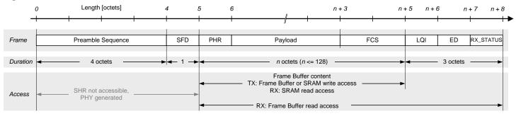
A frame comprises two sections, the radio transceiver internally generated SHR field and the user accessible part stored in the Frame Buffer. The SHR contains the preamble and the SFD field. The variable frame section contains the PHR and the PSDU including the FCS, see Section 8.3.
