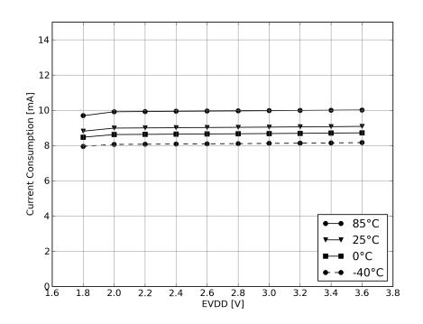
Figure 13-6. Current Consumption in RX\_ON State – Reduced Sensitivity.
