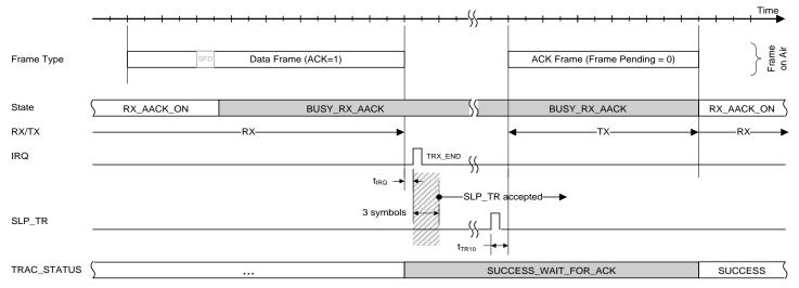
Figure 7-12. Timing Example of an RX\_AACK Transaction for Slotted Operation.
