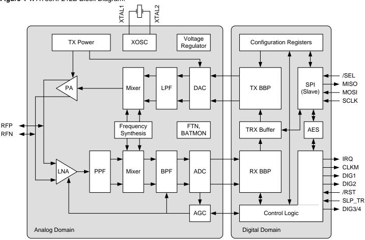
Figure 4-1. AT86RF212B Block Diagram.
