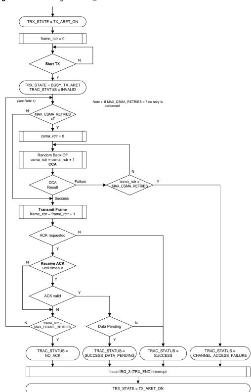
Figure 7-14. Flow Diagram of TX\_ARET.
