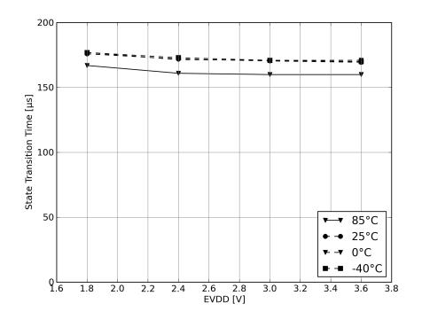
Figure 13-14. Transition Time from TRX\_OFF to PLL\_ON.
