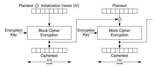
After preparing the AES key and defining the AES operation direction using Atmel AT86RF212B SRAM register bit AES\_DIR, the data has to be provided to the AES engine and the CBC operation can be started.
