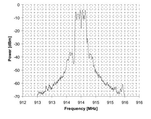
Figure 9-10. Spectrum of OQPSK-RC-100.
