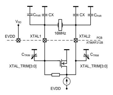
Additional internal trimming capacitors  $C_{\text{TRIM}}$  are available. Any value in the range from 0pF to 4.5pF with a 0.3pF resolution is selectable using XTAL\_TRIM of register 0x12 (XOSC\_CTRL). To calculate the total load capacitance, the following formula can be used
