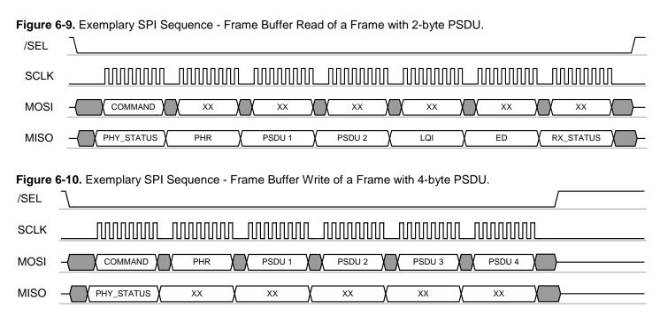
Access violations during a Frame Buffer read or write access are indicated by interrupt IRQ\_6 (TRX\_UR). For further details, refer to Section 9.4.
