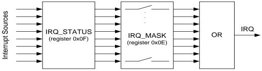
The Atmel AT86RF212B IRQ pin polarity can be configured with register bit IRQ\_POLARITY (register 0x04, TRX\_CTRL\_1). The default behavior is active high, which means that pin 24 (IRQ) = H issues an interrupt request.
