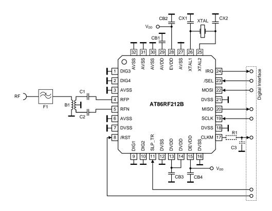
The power supply decoupling capacitors (CB2, CB4) are connected to the external analog supply pin 28 (EVDD) and external digital supply pin 15 (DEVDD). Capacitors CB1 and CB3 are bypass capacitors for the integrated analog and digital voltage regulators to ensure stable operation. All bypass capacitors should be placed as close as possible to the pins and should have a low-resistance and low-inductance connection to ground to achieve the best performance.
