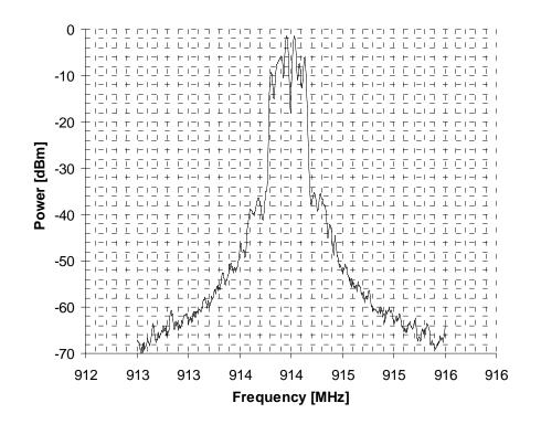
Figure 9-9. Spectrum of OQPSK-SIN-RC-100.
