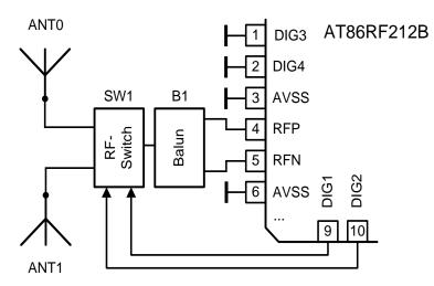
Figure 11-9. Antenna Diversity – Block Diagram.
