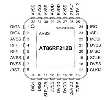
Figure 1-1. Atmel AT86RF212B Pin-out Diagram.
