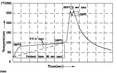
nmend pre-heat temperature of 105°C or less (as measured with a noccupie attached to the LED pins) prior to immersion in the solder with a maximum solder bath temperature of 260°C wave soldering temperature between  $245°C \sim 255°C$  for 3 sec (5 sec 1.Rec the wave 2.Peak
