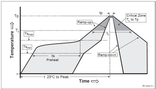
TCM 310 shall be handled according to Moisture Sensitivity Level MSL4 which means a floor time of 72 h. TCM 310 may be soldered only once, since one time is already consumed at production of the module itself.
