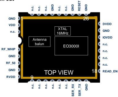
The figure above shows the pin out of the TCM 310x hardware.
