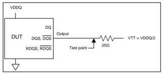
Output slew rate test load
