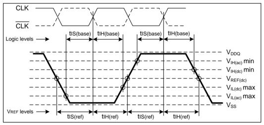
Figure 17 - Differential input waveform timing - tIS and tIH
