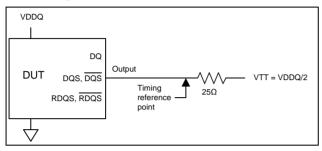
Figure 16 - AC timing reference load
