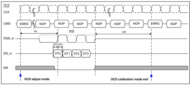
Figure 7 – OCD Adjust Mode
