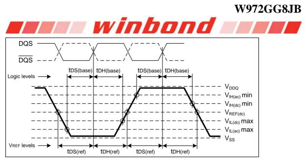
Figure 19 – Differential input waveform timing – tDS and tDH
