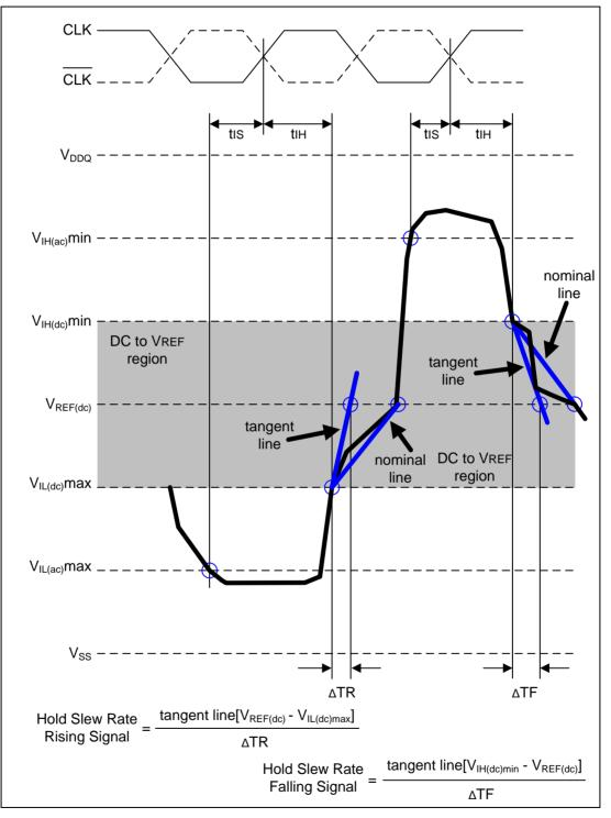
Figure 23 – Illustration of tangent line for till
