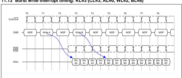
11.13 Burst write interrupt timing: RL=3 (CL=3, AL=0, WL=2, BL=8)
