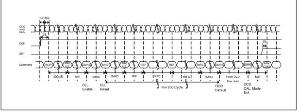
Figure 1 – Initialization sequence after power-up
