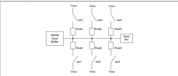
Switch (sw1, sw2, sw3) is enabled by ODT pin. Selection among sw1, sw2, and sw3 is determined by "Rtt (nominal)" in EMR (1). Termination included on all DQs, DM, DQS, DQS, RDQS, and RDQS pins. **Figure 9 – Functional Representation of ODT**
