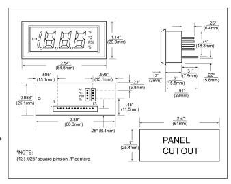
\*Note:Pins 2 & 4 should be tied together for proper operation.
