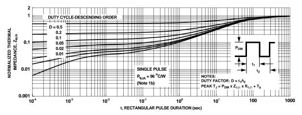
Figure 14. Transient Thermal Response Curve
