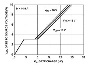
Figure 7. Gate Charge Characteristics
