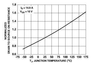
Figure 3. Normalized On-Resistance vs Junction Temperature
