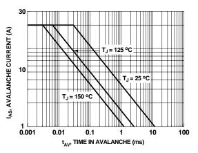
Figure 9. Unclamped Inductive Switching Capability
