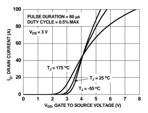
Figure 5. Transfer Characteristics
