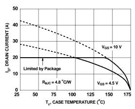
Figure 10. Maximum Continuous Drain Current vs Case Temperature
