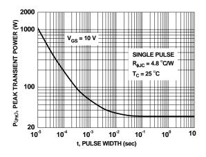
Figure 12. Single Pulse Maximum Power Dissipation
