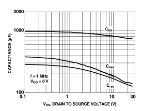
Figure 8. Capacitance vs Drain to Source Voltage
