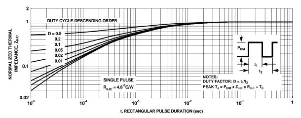
Figure 13. Transient Thermal Response Curve
