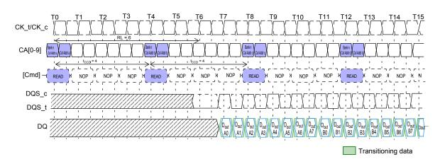
The seamless burst READ operation is supported by enabling a READ command at every fourth clock cycle for BL = 8 operation. This operation is supported as long as the banks are activated, whether the accesses read the same or different banks.
