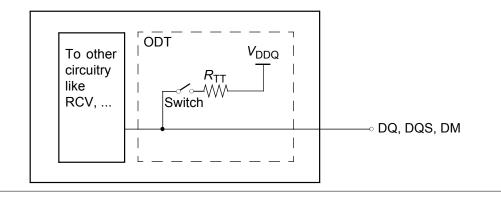
The switch is enabled by the internal ODT control logic, which uses the external ODT pin and other mode register control information. The value of RTT is determined by the settings of Mode Register bits. The ODT pin will be ignored if the Mode Register MR11 is programmed to disable ODT, in self-refresh, in deep power down, in CKE power down (mode register option) and during read operations.
