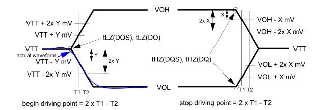
11. The parameters tLZ(DQS), tLZ(DQ), tHZ(DQS), and tHZ(DQ) are defined as single-ended. The timing parameters tRPRE and tRPST are determined from the differential signal DQS/DQS.
