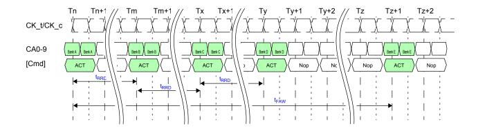
**Command Input Signal Timing Definition**
