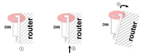
Figure 24: Removal of the DIN rail
