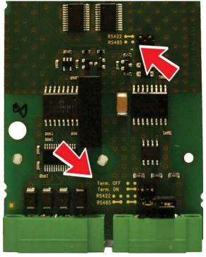
Figure 43: Connection of jumpers
