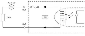
Figure 38: Binary output connection
