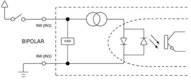
Figure 37: Binary inputs connection
