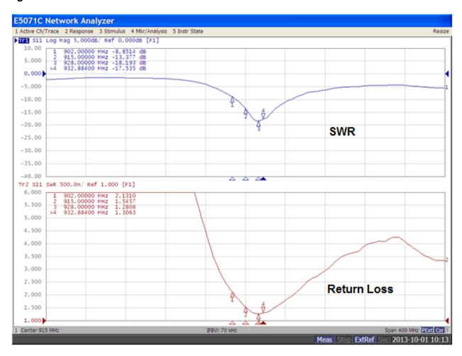
Figure 2 Typical Straight Position Reflection Performance
