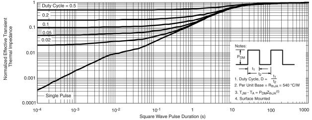
Normalized Thermal Transient Impedance, Junction-to-Ambient
